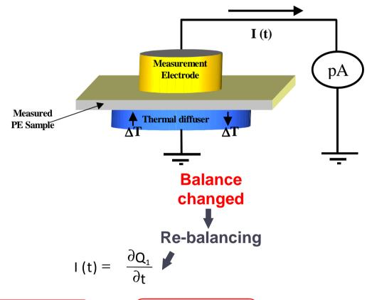
$$I(t) = -\alpha \ C \int_{0}^{D} E(x) \frac{\partial \Delta T(x,t)}{\partial t} dx \qquad \Longrightarrow \left(\rho(x) = \epsilon \frac{\partial E(x)}{\partial x}\right)$$
